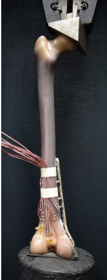
Figure 3. Biomechanical testing setup with strain gauges attached to the posterior distal femur at locations of greatest stress concentration as determined by photostress analysis.
