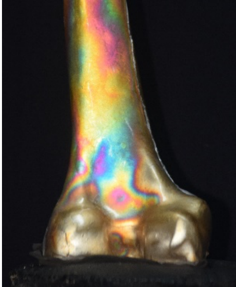
Figure 2. Photostress analysis, with locations of greatest color gradient corresponding to locations of greatest stress within the posterior distal femur.
