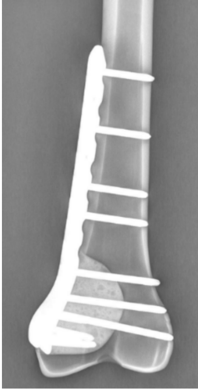
Figure 1. Anteroposterior radiograph of a composite left distal femur, status post creation of a contained medial distal femur defect, cementation, and placement of an 8-hole medial distal femur locking plate.
